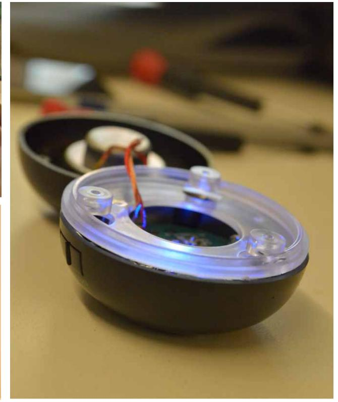
The prototype was constructed in Solidworks and then was cnc milled in two shells. The resulting product created an oscillation chamber which when paired with a speaker created a device that would sync your sense of touch and hearing to enhance focus while in meditation.
